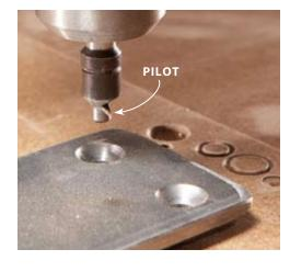
3 Using the same bit you used for the pilot holes, position the plate and drill through it just enough to make a small dimple in the wood you'll be fastening it to.
