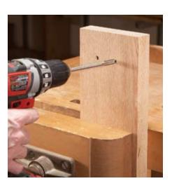
8 I prefer to use machine screws that have an Allen head. To make assembly easier, I insert the screws with a driver made by cutting off the end of an Allen wrench.
