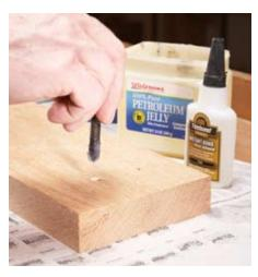
5 Chuck the tap into a drill, set the drill at low speed, and run the tap through the hole. The drill won't wobble—the tap's long, tapered snout will guide it straight through the hole.
