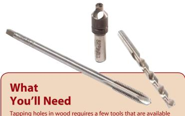
from an industrial supply house. The most important tool is the tap. I've found that a special tap with an undercut shank and a long, tapered point works best. (See Source, page 45, for supplies for 1/4-20 screws; supplies for 5/16-18 and other screws are also available here.)
