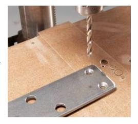
**2** To ensure that the countersink in each hole is perfectly centered, re-drill them using a piloted countersink bit. The pilot's diameter must match the drill bit you used above.
