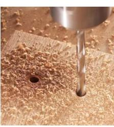
**7** For hard use, strengthen the threads in the wood with CA glue. Dribble glue in the hole, then insert a machine screw coated with petroleum jelly. After the glue cures, remove the screw.
